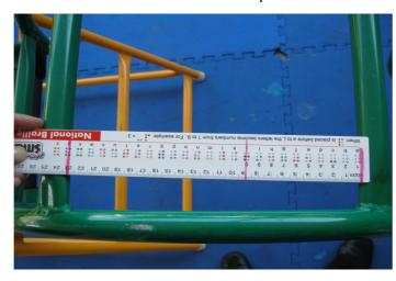
A ruler or tape measure could be used to check for bound head and neck entrapment hazards in the set up of fixed and mobile equipment (example pictured above).
